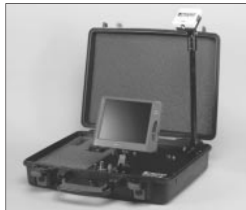
BCR-100 Briefcase Receiver used with High Power Transmitter for Covert Applications
